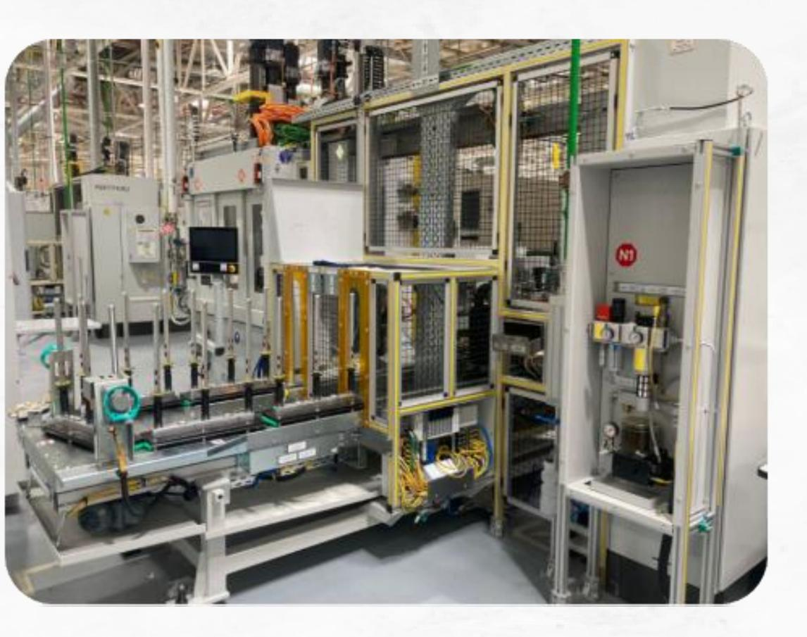
FELSOMAT AUTOMATION FOR NAGEL HYBRID MACHINE Integration and redesign to load and unload gears to Nagel honing machine at Ford sun gears area.
