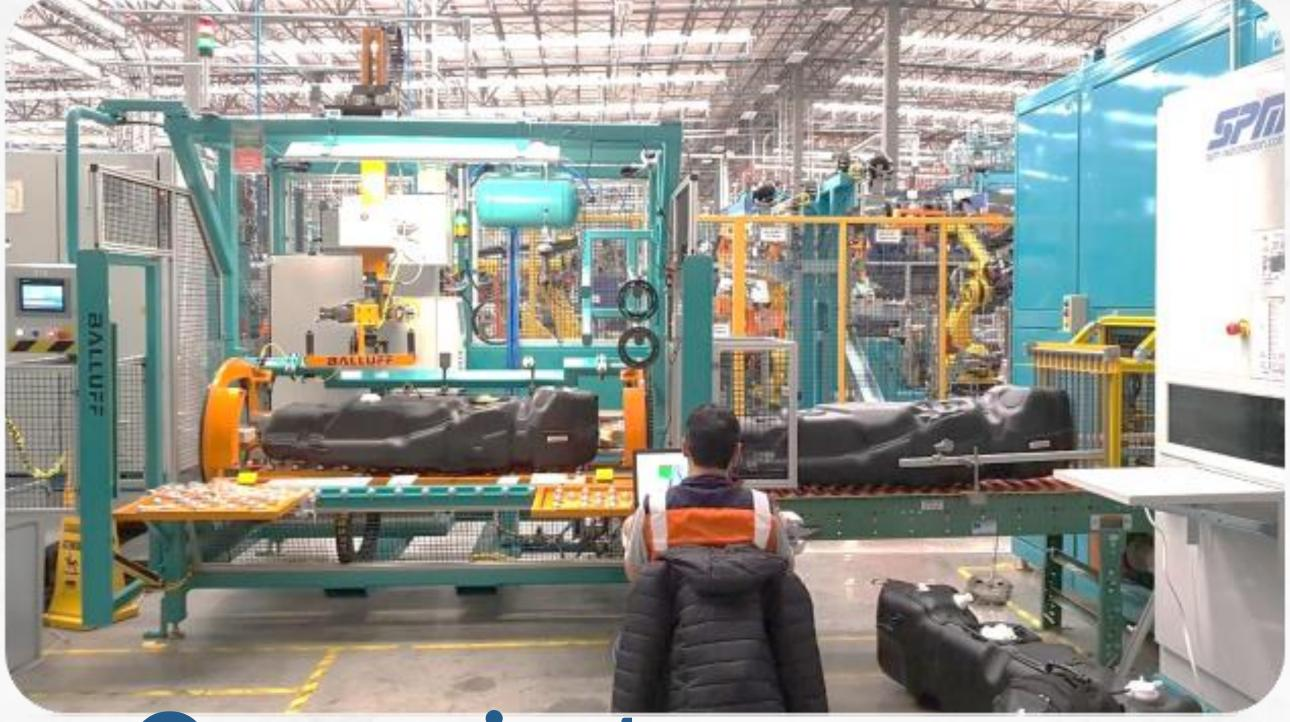
Automatic station for fuel pump installation and continuity test
