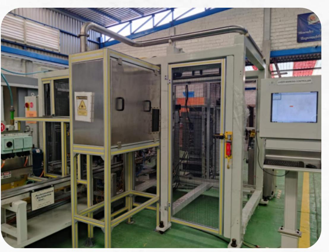
Design manufacturing and Integration of a telesis laser marker, dataman 2D reader and an ASI automation for a shot peening machine.
